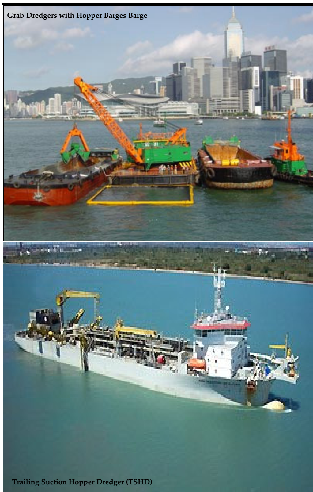
Figure 10.11 Grab Dredgers with Hopper Barges Barge and Trailing Suction Hopper Barge
