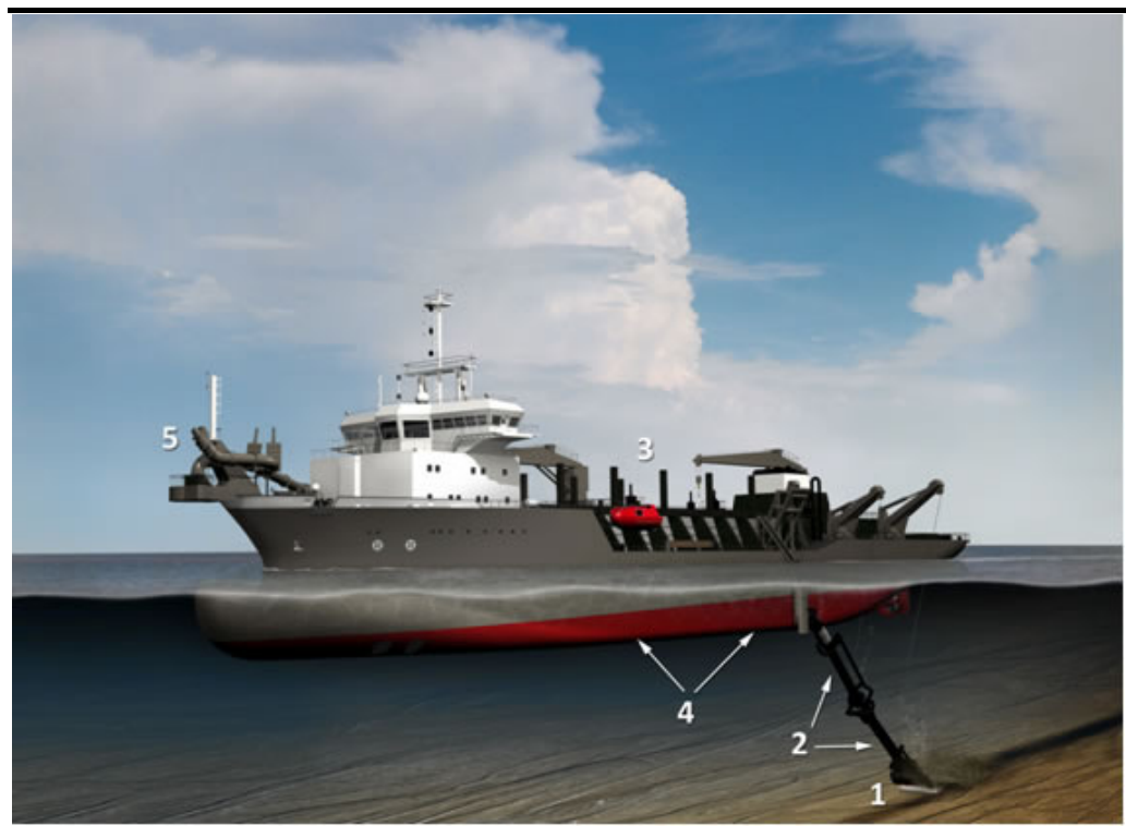
Figure 3.2 Trailing Suction Hopper Dredger (TSHD)
