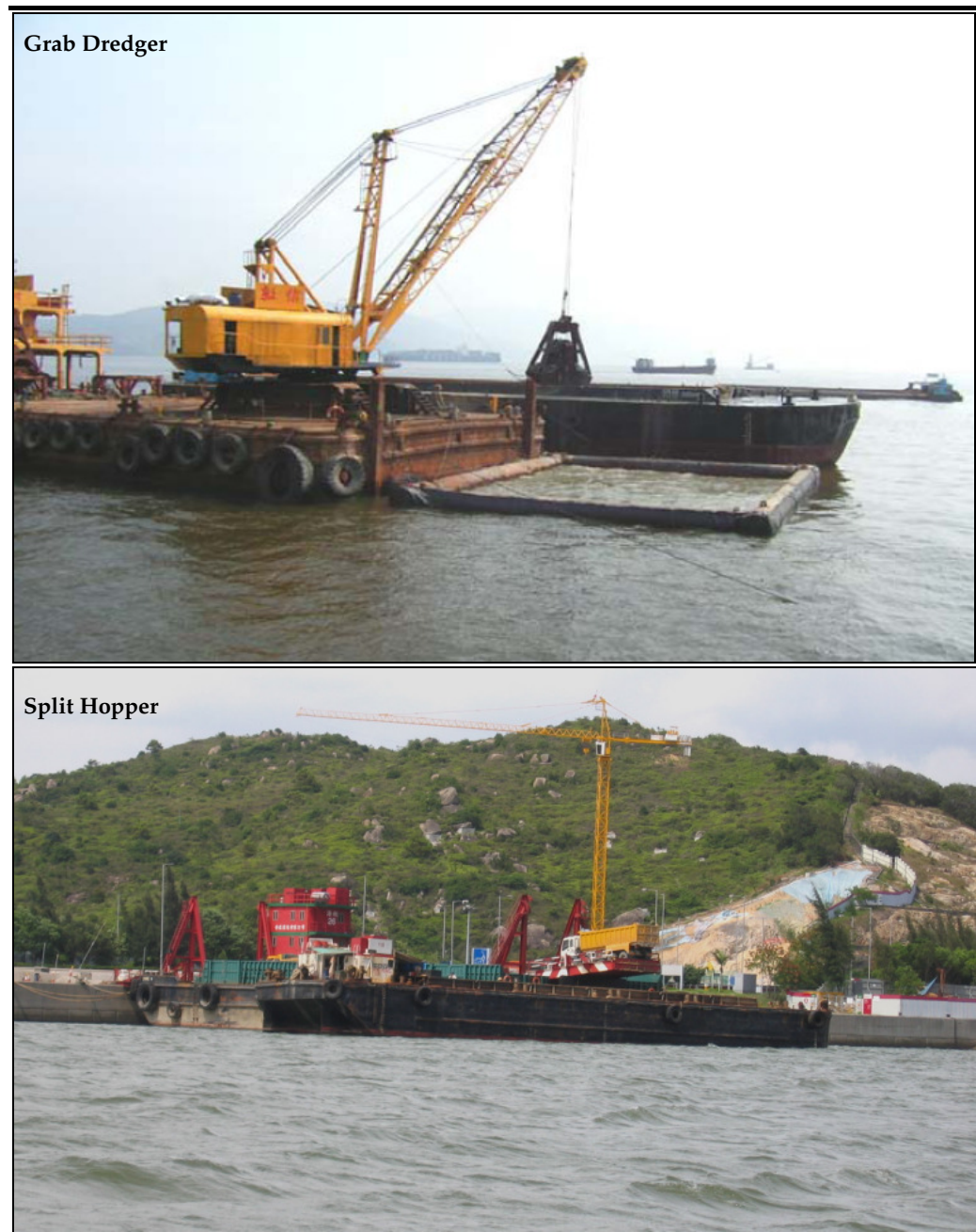
Figure 10.10 Grab Dredger and Split Hopper
